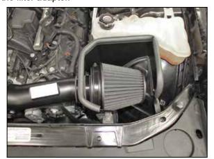
23. Install the filter assembly onto the K&N® intake tube and secure with the provided hose clamp.
