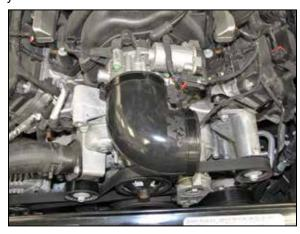
14. Install the provided 90° coupling hose (084088) onto the throttle body and secure with the provided hose clamps
