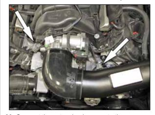
20. Connect the extension harness to the factory engine harness and then into the inlet air temperature.
