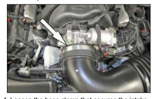
4. Loosen the hose clamp that secures the intake hose to the throttle body and then pull the intake tube from the throttle body.
