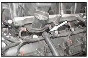
5. On models equipped with a 5.7L. Disconnect the crank case vent hose from the valve cover port.
